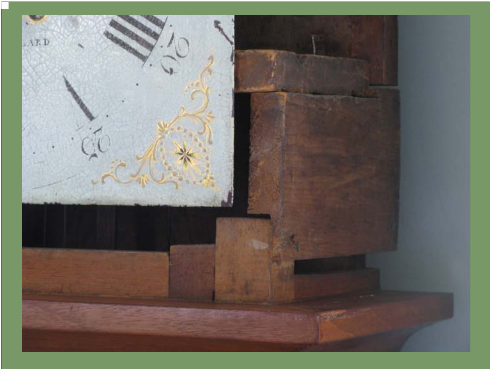
Number 2 – Support blocks for the works are rabbeted into the upper ends of the case sides.
